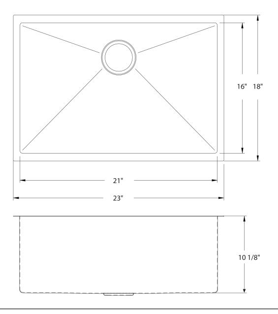
**ATTENTION!** Dimensions may vary by up to 3/8". It is highly recommended to pull all dimensions of actual model for installation and measuring purposes.
